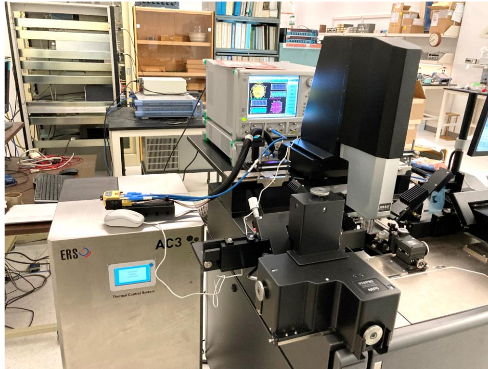
220 GHz 2 port installation at NIST on MPI semi-automatic TS2000-THZ station
