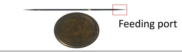
Dielectric rod waveguide(DRW)
