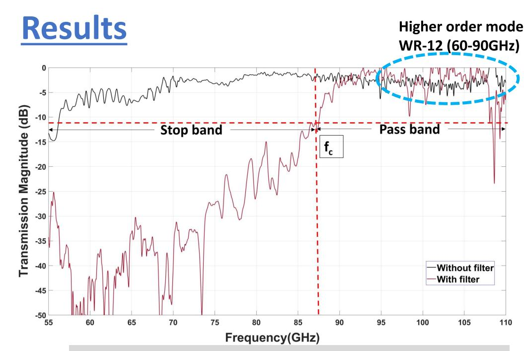
Attenuated low frequency > working High pass filter
