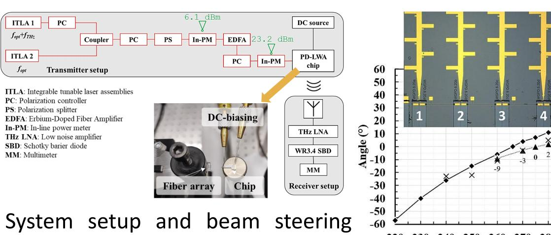
System setup and beam steering characterization at WR3.4 band
